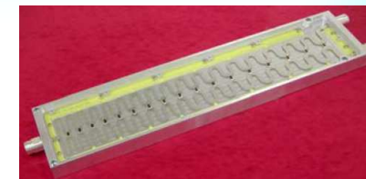
Ultra wideband 70 to 2700 MHz Wilkinson Divider/Combiner using 17 sections with an air dielectric for minimum loss
