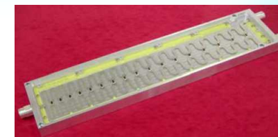
Ultra wideband 70 to 2700 MHz Wilkinson Divider/Combiner using 17 sections with an air dielectric for minimum loss
